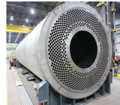
Gas-Gas Heat Exchanger
