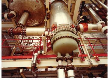
delivered to satisfied clients around the globe. Completed plants range in capacity from **25 to 2200 MTPD** and concentrate sulphuric acid from a starting concentration as low as 7 wt% to product concentrations between 83-96 wt% sulphuric acid.
