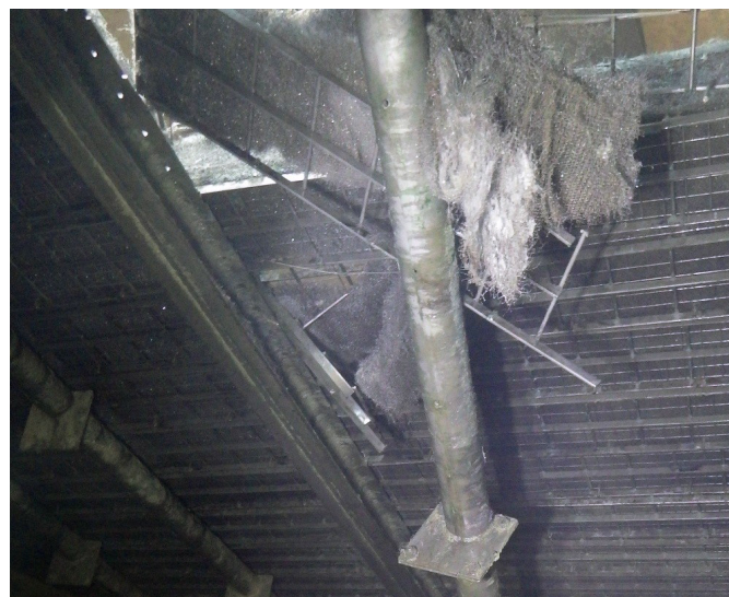
Common mechanical failure as seen on competitors' historical mesh pad designs within 1 or turnaround cycle (catastrophic failure)
