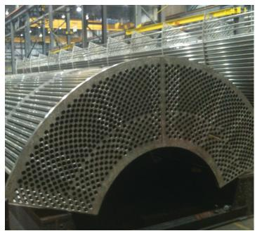
Transferring large quantities of heat from one gas stream to another using gas to gas heat exchangers is essential to the process of manufacturing sulphuric acid. With over 400 units installed since the Worley Chemetics (Chemetics®) development and patent in 1978, we have specialized in the design, engineering and fabrication of Gas to Gas Heat Exchangers.
