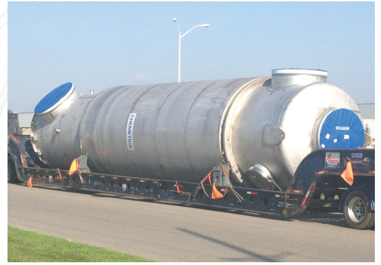
Preheat Exchangers fully fabricated and shippable to site
