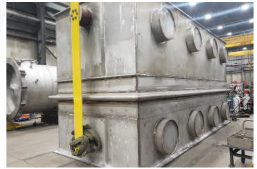
CORE TM Tube Bundle Ready for Shipment
